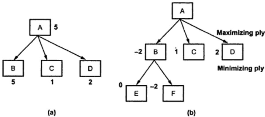
Suppose node B is examined one more level as shown in fig B. then we see because of a minimizing ply value at B is -2 and hence the value passed to A is 2. This results in a drastic change in the situation. There are two proposed solutions to this problem, neither very satisfactory.
