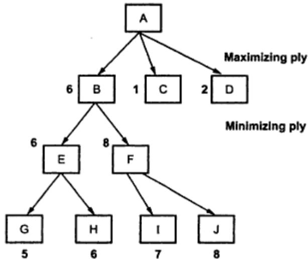
Fig above shows the further exploration of the tree in fig B. Here now since the tree is further explored, the value, which is passed to A is 6. Thus the situation calms down. This is called as waiting for quiescence. This helps in avoiding the horizon effect of a drastic change of values.
